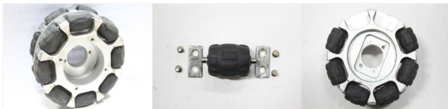
Fig. 3. Left: the new Omni-directional Wheel. Middle: Roller. Right: Wheel hub
